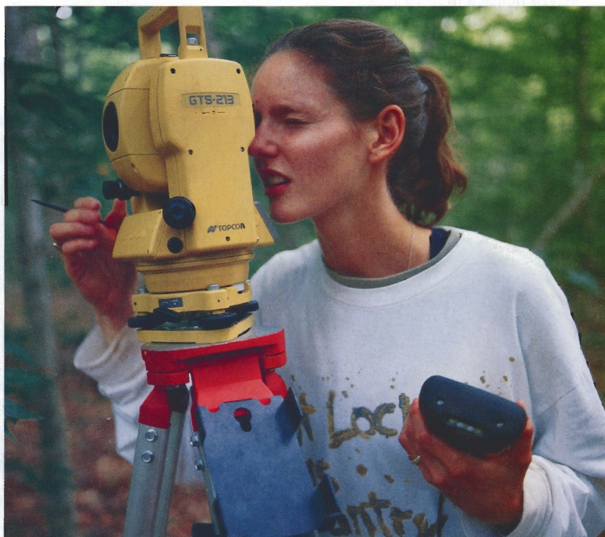
Student Melissa Smith uses a laser transit to map rock fences, foundations, stone enclosures, and topographic features. The laser transit gathers very precise distance and elevation measurements.
